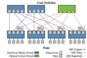
Figure 1: Helios is a 3-level multi-rooted tree of pod switches and core switches. The core consists of both traditional electrical packet switches and MEEMS-based optical circuit switches. Superlinks are defined in §3.1.
