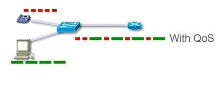
ip access-list extended QOS-LOW-LATENCY-DATA remark Latency sensitive Data application traffic permit tcp host 10.1.1.2 any any permit tcp host 10.1.1.4 any any deny ip any any
